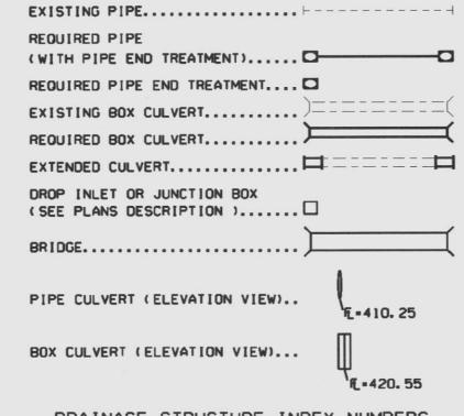
DRAINAGE STRUCTURE INDEX NUMBERS DRAINAGE STRUCTURE WRITE-UPS ARE LOCATED ON THE DRAINAGE CROSS-SECTION SHEETS. STRUCTURES WITH WRITE-UPS ARE INDEXED AT EACH END. WITH NUMBERS ASSIGNED BY DIRECTION OF FLOW. THE NUMBER IN THE UPPER HALF OF THE CIRCLE (EXAMPLE 8 OR 9) IS THE DRAINAGE STRUCTURE INDEX NUMBER. THE NUMBER IN THE LOWER HALF (EXAMPLE 88) IS THE SHEET REFERENCE NUMBER.
